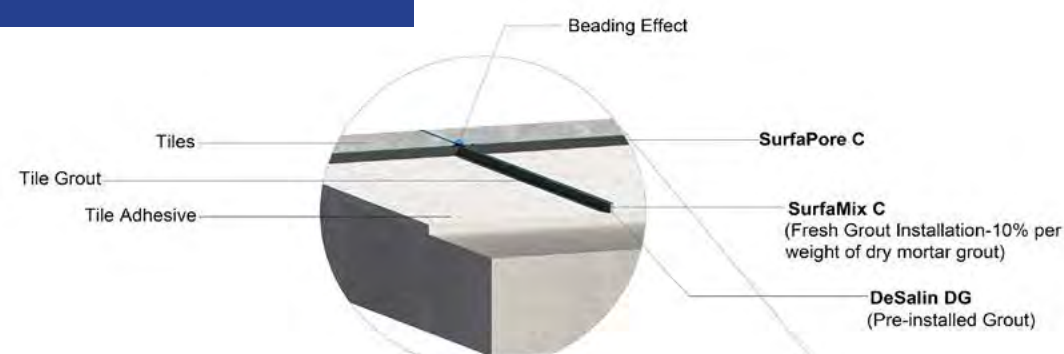
The beading effect on grout is intense, even if the grout gap is huge.
