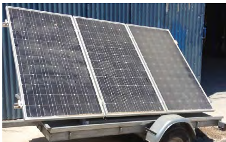
Anti-dust performance of SurfaShield G coated panels: two left panels have been treated with SurfaShield G, while the right one remains untreated for six months in Cyprus. Note the accumulation of dust in the aluminium base of the panels.
