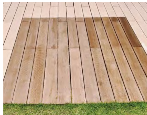
Application of a single SurfaPaint HDO coat on wooden composite deck flooring. Upper right application corner has been treated with an extra SurfaPaint HDO coat. Photo is taken 12 months after application on a sample applied next to coastline area and subjected to desert heat/irradiation.
