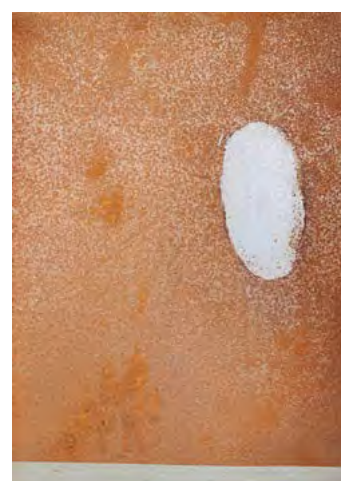
Final result of rust removal, within 10min of DeSalin Gel Rust Remover application.
