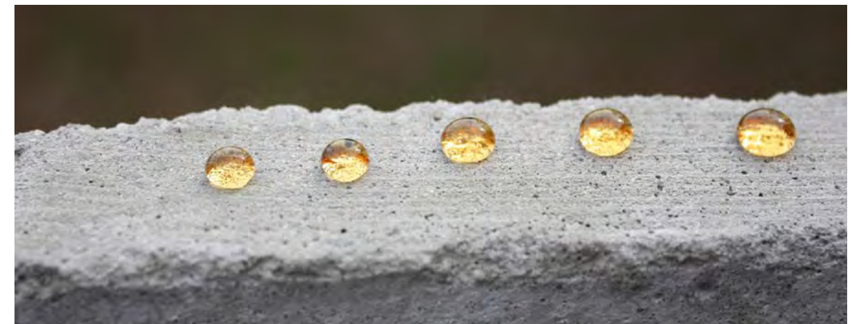
Oil droplets on a SurfaPore M treated porous, cementitious surface.
