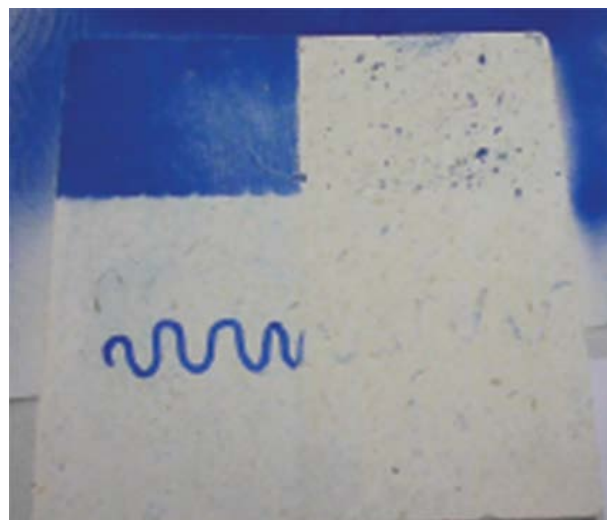
Anti-graffiti effect on a porous surface. Right half-side is SurfaPore AG and subjected to cleaning under hot-water, without scrubbing.
