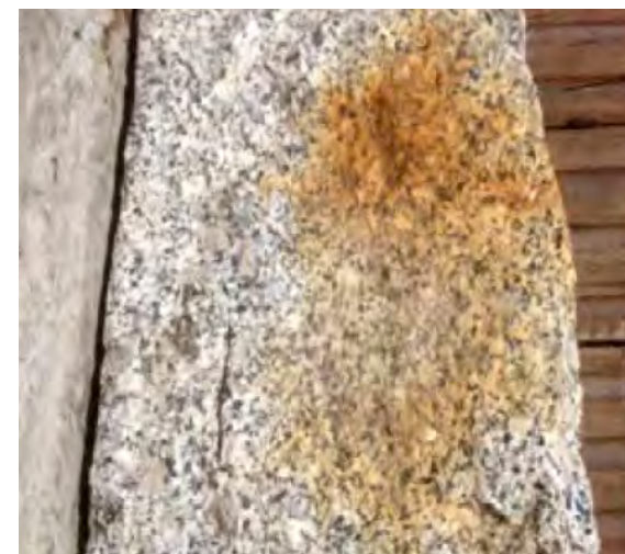
Rust deposits on a chemicals-resistant granite piece.
