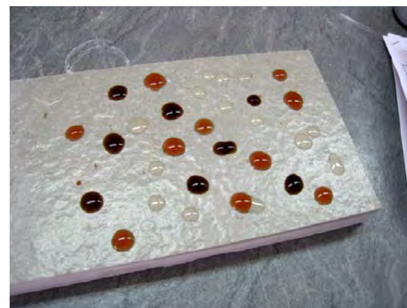
Staining (left) and cold-water cleaning (right) of a natural stone tile treated with SurfaPaint Stone Varnish WB.
