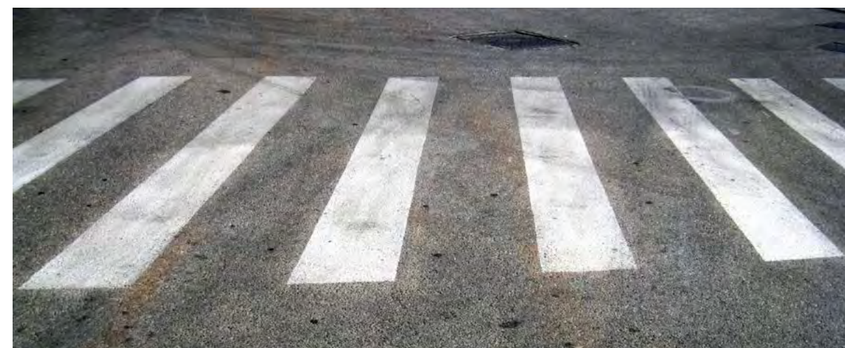
The effect of SurfaShield C on a heavy-traffic pedestrian zebra crossing, three months after treatment. Upper side is the original road traffic paint, while the lower part has been treated with SurfaShield C.
