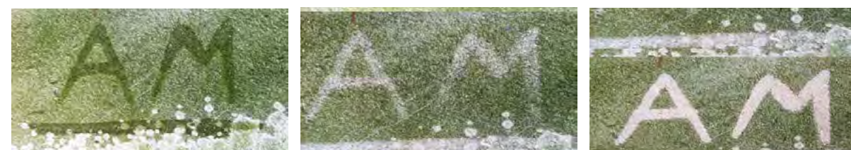
The application of DeSalin AM on a mouldy surface, immediately, after 24h and after 10 days from application.
