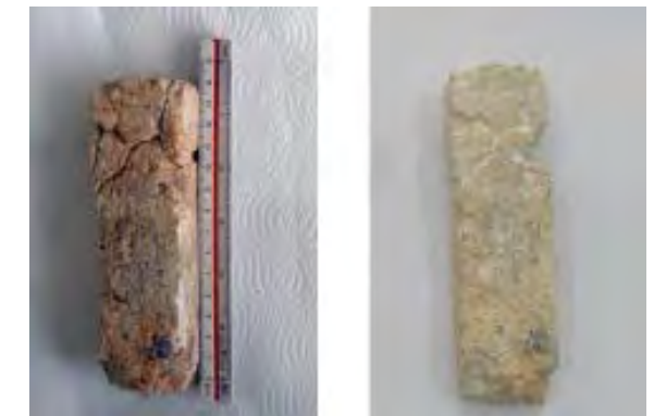
Egyptian Calcite sandstone sample before treatment (left) and after treatment (right).
