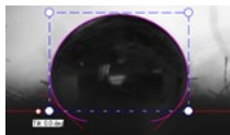
Oil droplet on SPH treated fabric Contact angle _{0\text{ min}}=136.78 Contact angle _{5\text{ min}}=124.94^\circ
